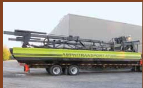
The Amphittransport is equipped with four articulated hydraulic anchor piles which make it possible to work with total stability. The AT 300 moves at a speed of 5 to 8 knots with powerful hydraulic engine propellers. It also moves from the bank to the water without external assistance thanks to these articulated anchor piles.
